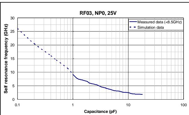
Fig. 5 Self resonance frequency vs. Capacitance (0201 size)
