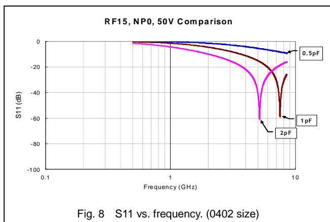
Fig. 8 S11 vs. frequency. (0402 size)
