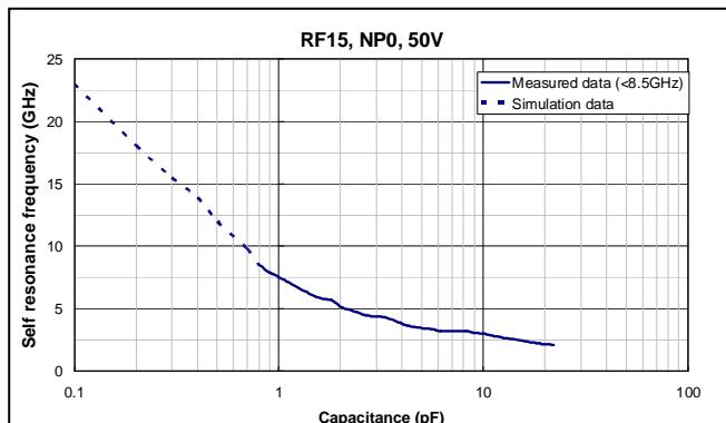
Fig. 6 Self resonance frequency vs. Capacitance (0402 size)
