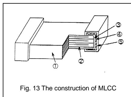
Fig. 13 The construction of MLCC
