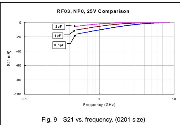
Fig. 9 S21 vs. frequency. (0201 size)
