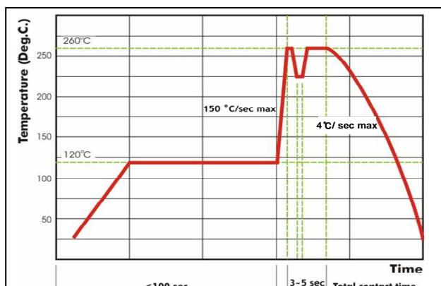
Fig. 15 Recommended wave soldering profile for SMT process with SnAgCu series solder.
