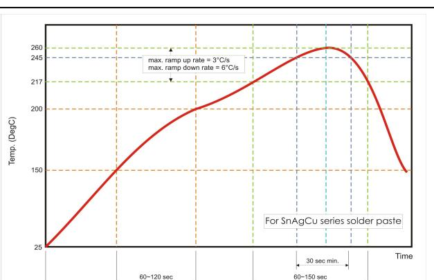
Fig. 14 Recommended reflow soldering profile for SMT process with SnAgCu series solder paste.
