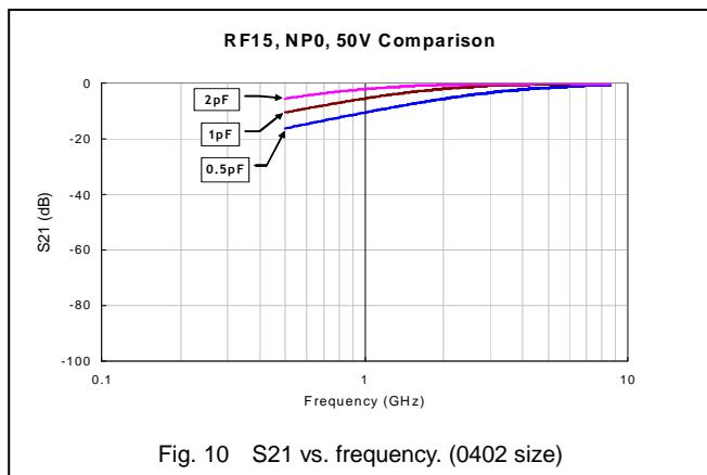
Fig. 10 S21 vs. frequency. (0402 size)
